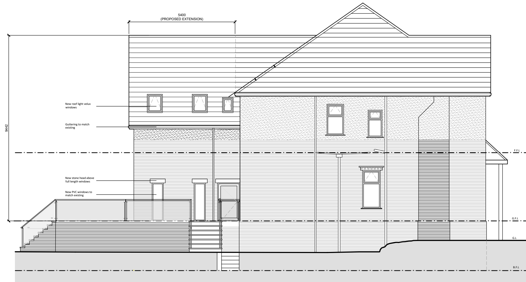
Proposed Side Elevation- 1 : 50
